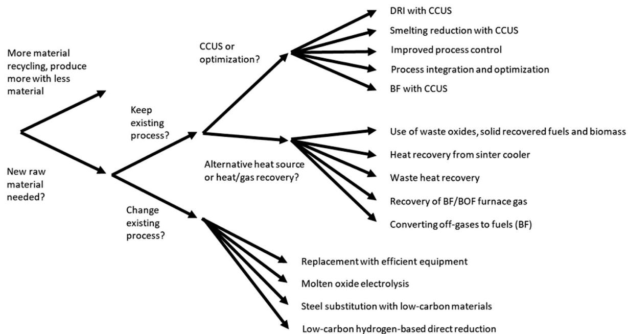
**Fig. 16.** Decision tree of decarbonization choices for the iron and steel industry.
