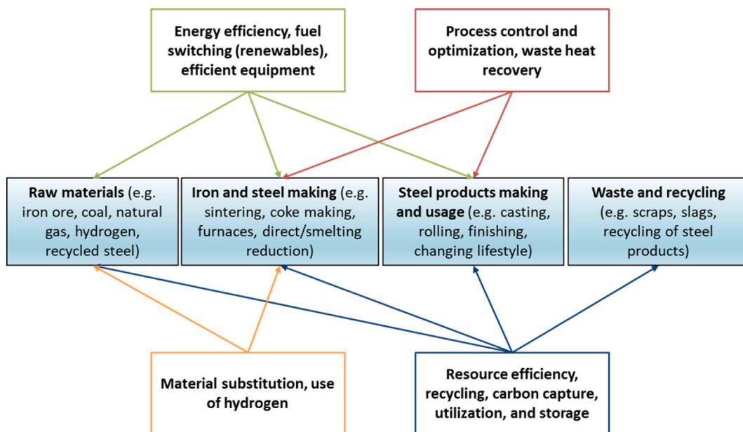
**Fig. 26.** Visualizing crosscutting options for the decarbonization of the iron and steel system.
