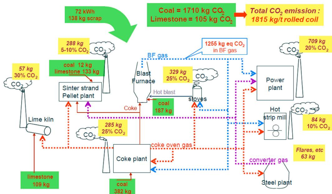
**Fig. 8.** CO<sub>2</sub> emissions from a typical steel mill.
