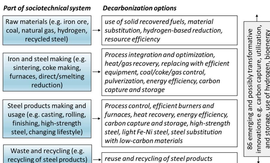
**Fig. 11.** Sociotechnical options for decarbonizing the iron and steel industry.
