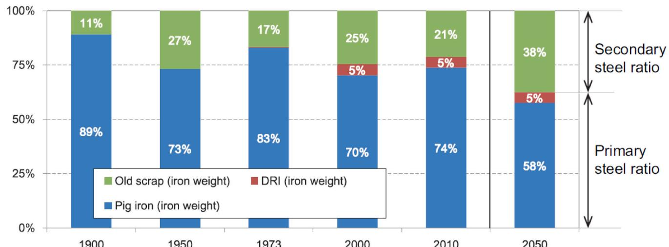
Fig. 15. Steel scrap recycling and the expansion of secondary steel.
