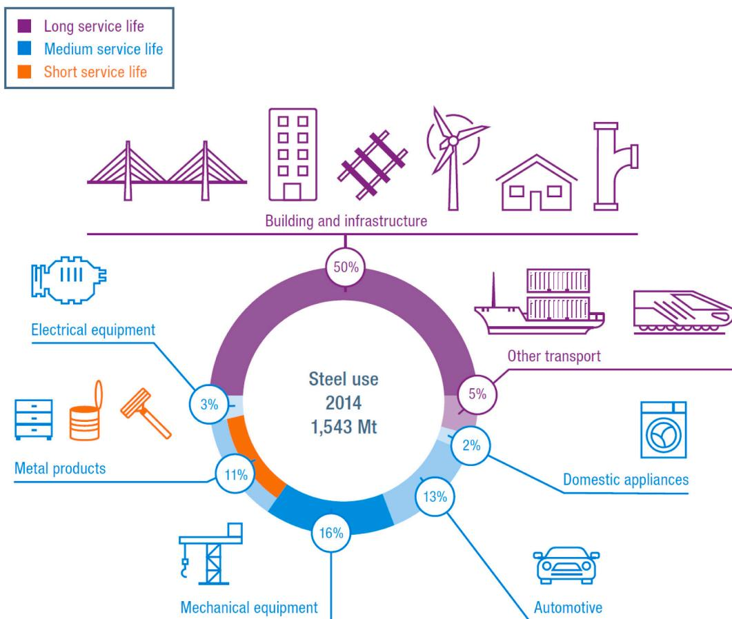
Fig. 24. Steel products and durability.
