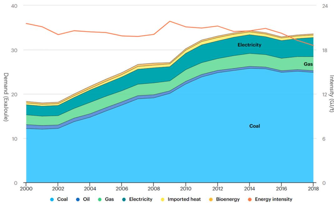
**Fig. 1.** Energy demand and intensity of the global iron and steel industry (2000–2018).
