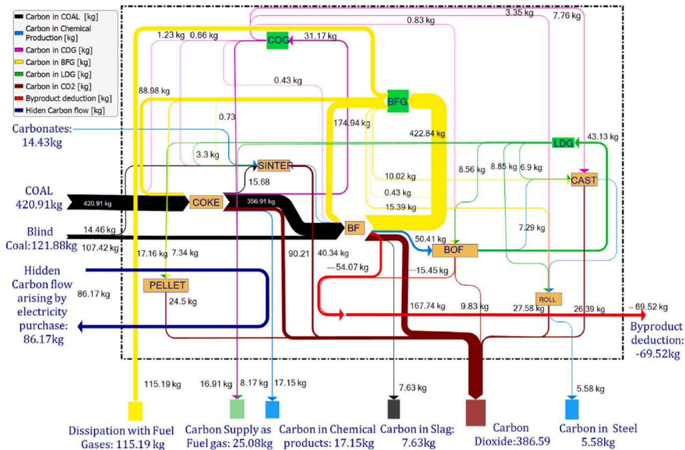
Fig. 13. A carbon flow chart for BF/BOF steel processing.
