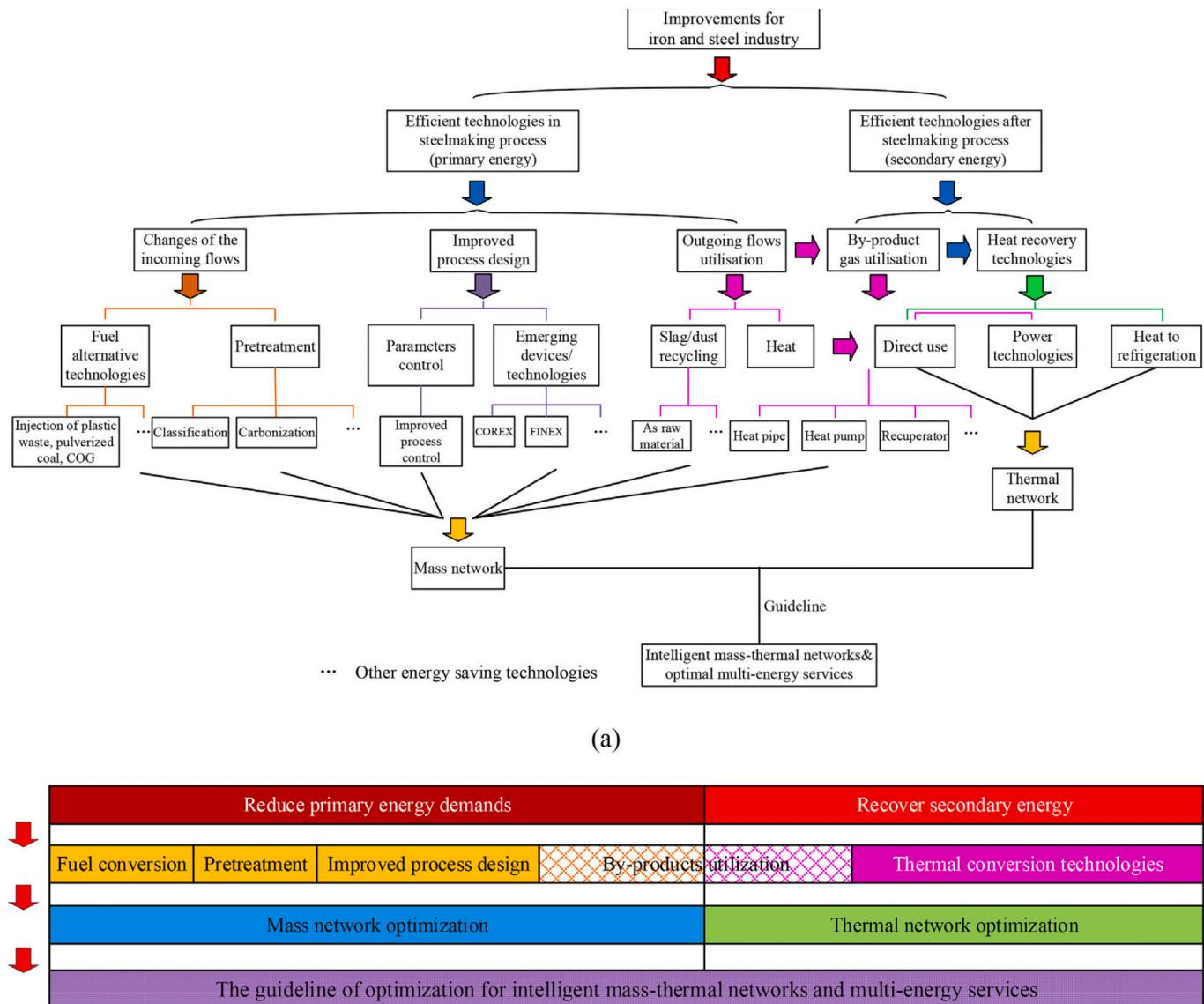
**Fig. 14.** Roadmap of efficient use of energy in iron and steel industry (top panel (a): main concepts, bottom panel (b): general summarization).
