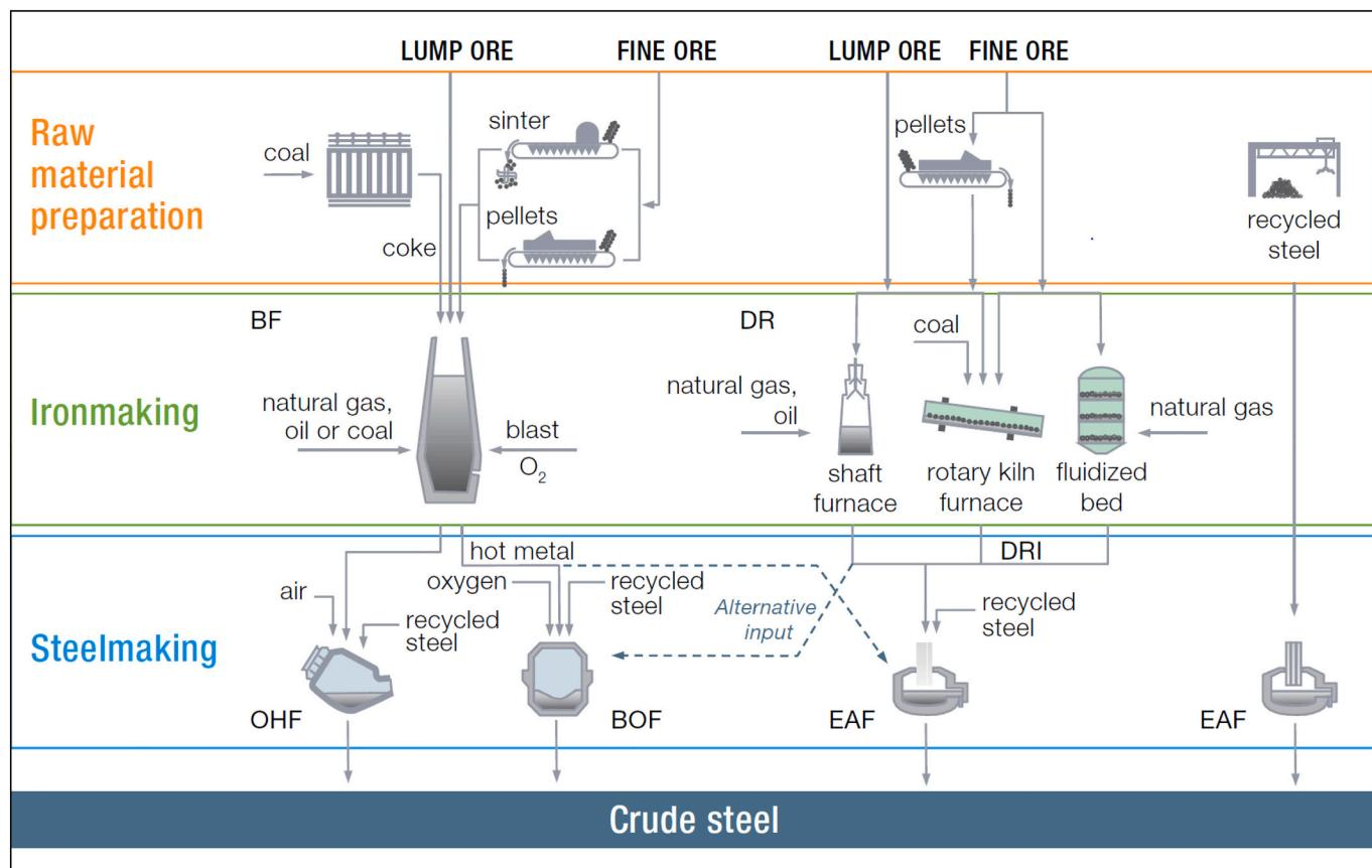
Fig. 2. Iron and steelmaking routes.
