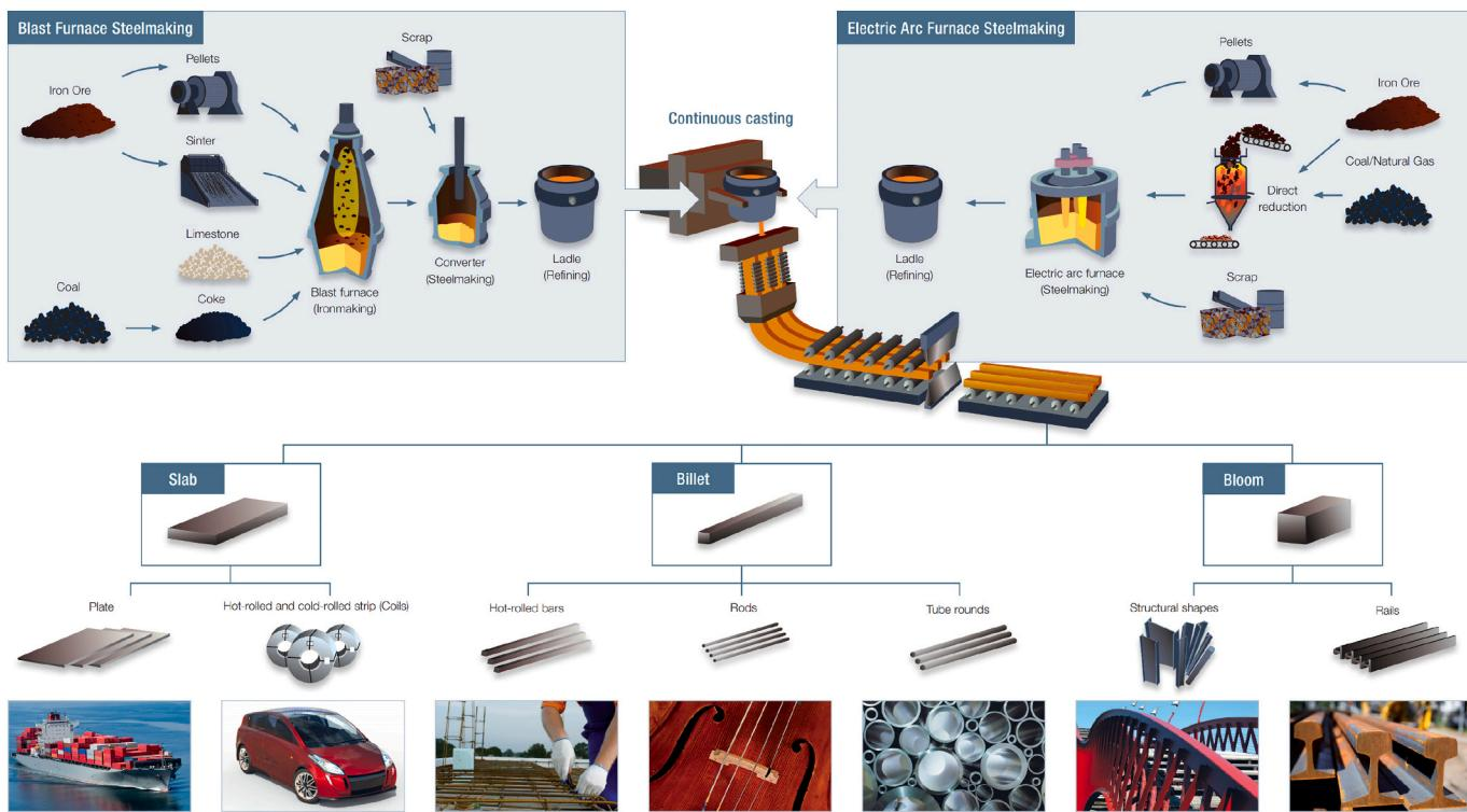
Fig. 3. Iron and steelmaking routes.
