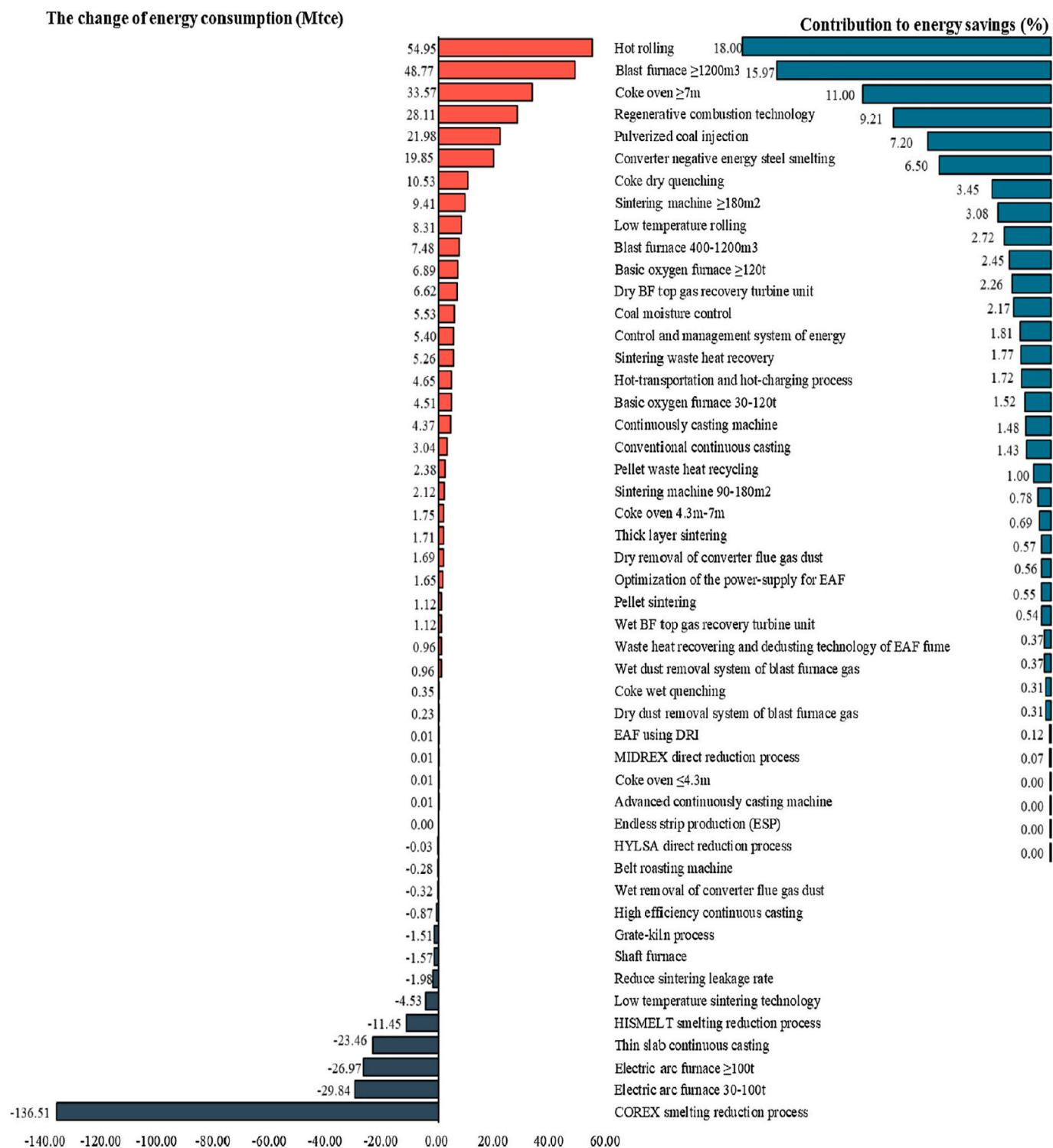
Fig. 20. Energy savings contributed by each technology in China's iron and steel industry.
