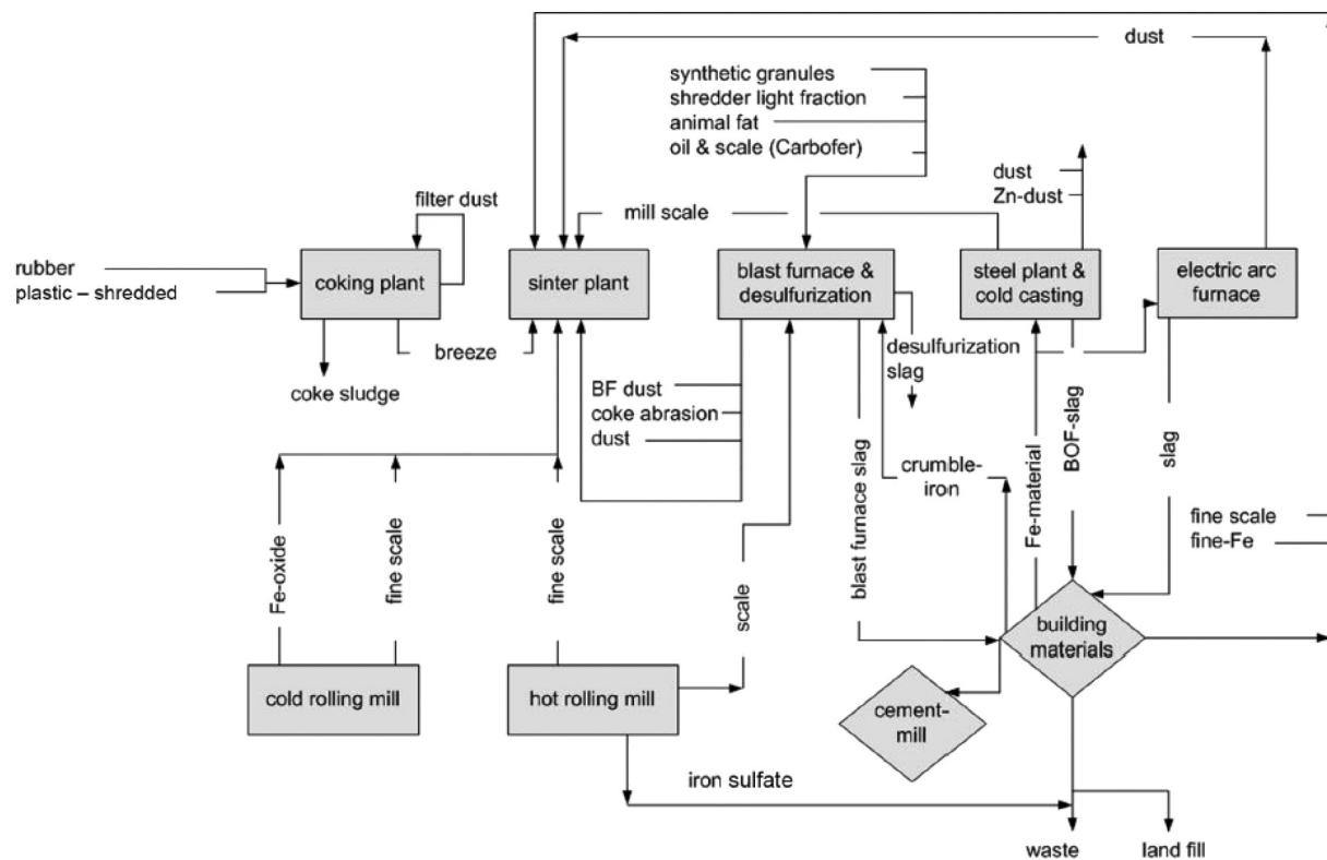
**Fig. 12.** Recycling of waste materials for a metallurgical plant.
