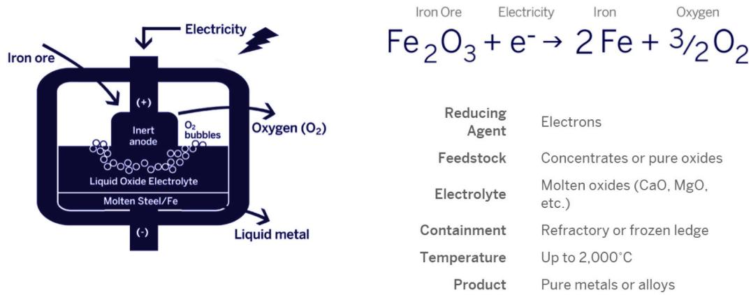
**Fig. 19.** Molten oxide electrolysis.
